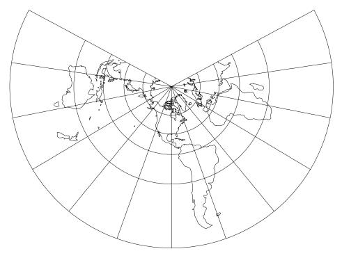
Figure 37: Lambert Conformal Conic projection, with shorelines and 30° graticule. Central Meridian 90° W. and standard parallels at 20° N and 60° N (+proj=lcc +lon\_0=90w +lat\_1=20n +lat\_2=60n).
