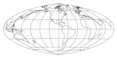
Figure 55: Eckert-Greifendorff modified Hammer projection, with shorelines and 30° graticule. Central Meridian 90° W. (+proj=hammer +lon\_0=90w +W=.25)
