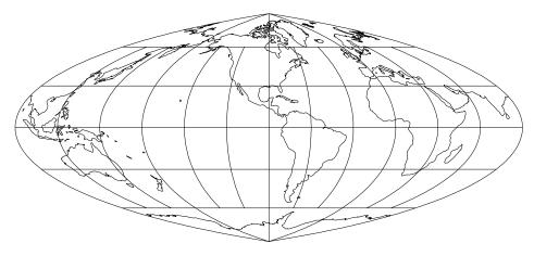
Figure 31: Quartic Authalic projection, with shorelines and 30° graticule. Central Meridian 90° W (+proj=quau +lon\_0=90w).
