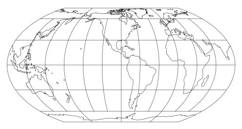
Figure 29: Putninš  $P'_2$  projection, with shorelines and 30° graticule. Central Meridian 90° W (+proj=putp2 +lon\_0=90w).
