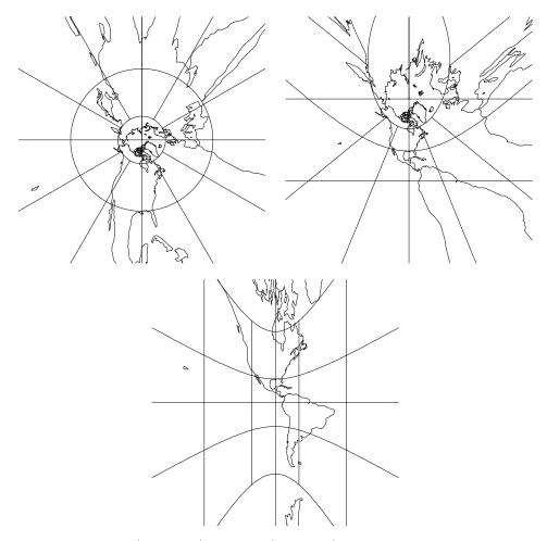
Figure 48: Polar (lat\_0=90), oblique (lat\_0=45) and equatorial aspects of the Gnomonic projection, with shorelines and 30° graticule. Central Meridian 90° W. (+proj=gnom +lon\_0=90w)
