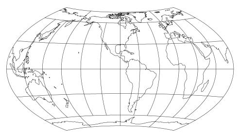
Figure 56: Wagner VII projection, with shorelines and 30° graticule. Central Meridian 90° W. (+proj=wag7 +lon\_0=90w)
