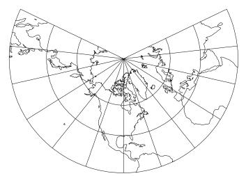
Figure 39: Perspective Conic projection, with shorelines and 30° graticule. Central Meridian 90° W and standard parallels at 20° N and 60° N (+proj=pconic +lon\_0=90w +lat\_1=20n +lat\_2=60n).
