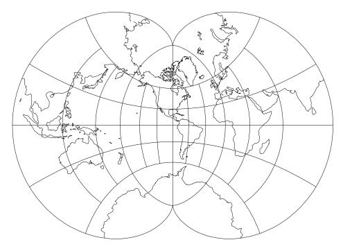
Figure 59: August Epicycloidal projection, with shorelines and 30° graticule. Central Meridian 90° W (+proj=august +lon\_0=90w).
