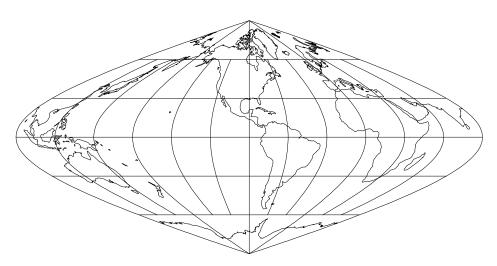
Figure 30: Putninš P<sub>5</sub> projection, with shorelines and 30° graticule. Central Meridian 90° W (+proj=putp5 +lon\_0=90w).
