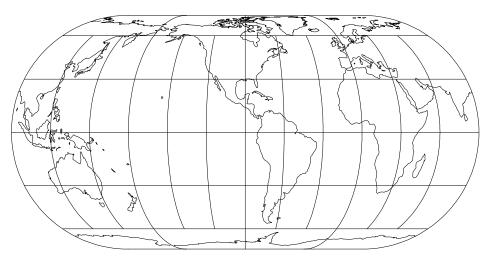
Figure 20: Eckert IV projection, with shorelines and 30° graticule. Central Meridian 90° W (+proj=eck4 +lon\_0=90w).
