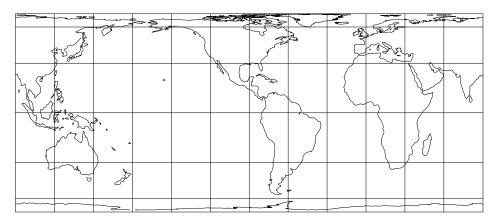
Figure 7: Behrmann Equal Area projection, with shorelines and 30° graticule. Central meridian 90° W. Standard parallels 30° (+proj=cea +lon\_0=90w +lat\_ts=30).
