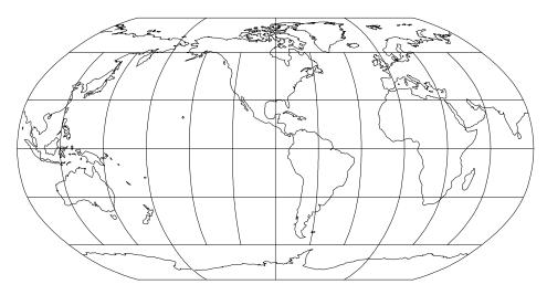
Figure 16: Robinson projection, with shorelines and 30° graticule. Central Meridian 90° W (+proj=robin +lon\_0=90w).
