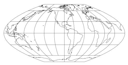
Figure 26: McBryde-Thomas Flat-Polar Parabolic projection, with shorelines and 30° graticule. Central Meridian 90° W (+proj=mbtfpp +lon\_0=90w).
