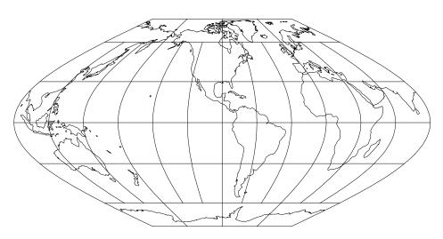
Figure 28: McBryde-Thomas Flat-Polar Sinusoidal projection, with shorelines and 30° graticule. Central Meridian 90° W (+proj=mbtfps +lon\_0=90w).
