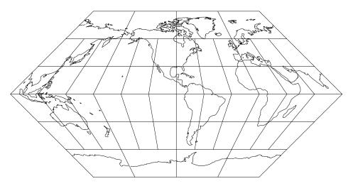
Figure 17: Eckert I projection, with shorelines and 30° graticule. Central Meridian 90° W (+proj=eck1 +lon\_0=90w).
