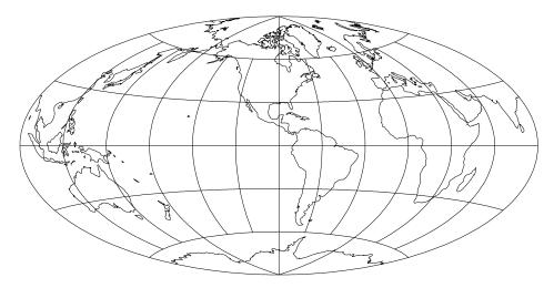
Figure 57: Aitoff projection, with shorelines and  $30^{\circ}$  graticule. Central Meridian  $90^{\circ}$  W. (+proj=aitoff +lon\_0=90w)
