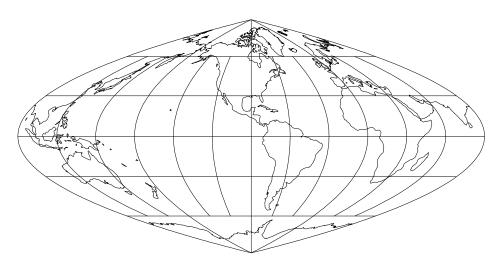
Figure 36: Craster Parabolic projection, with shorelines and 30° graticule. Central Meridian 90° W (+proj=parab +lon\_0=90w).
