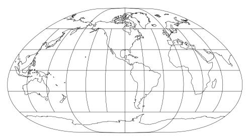
Figure 25: Loximuthal projection, with shorelines and 30° graticule. Central Meridian 90° W (+proj=loxim +lon\_0=90w +lat\_1=40n).
