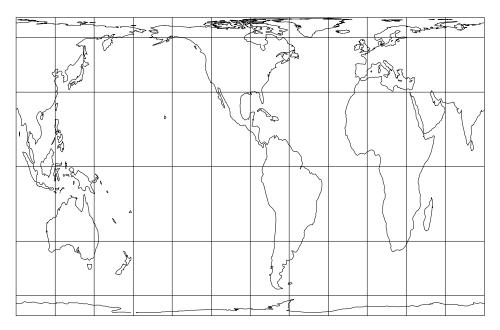
Figure 8: Gall's Orthographic or approximate Peters projection, with shorelines and 30° graticule. Central meridian 90° W. Standard parallels 45° (+proj=cea +lon\_0=90w +lat\_ts=45).
