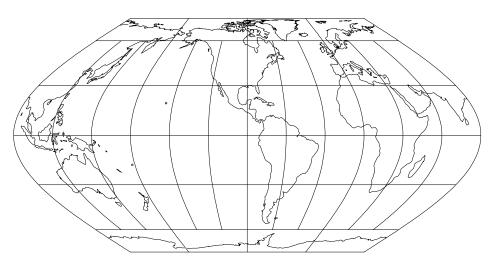
Figure 22: Eckert VI projection, with shorelines and 30° graticule. Central Meridian 90° W (+proj=eck6 +lon\_0=90w).
