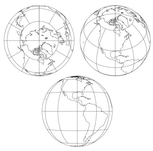
Figure 51: Polar (lat\_0=90), oblique (lat\_0=45) and equatorial aspects of the Near-Sided Perspective projection, with shorelines and 30° graticule. Central Meridian 90° W. (+proj=nsper +lon\_0=90w +a=1 +h=8)
