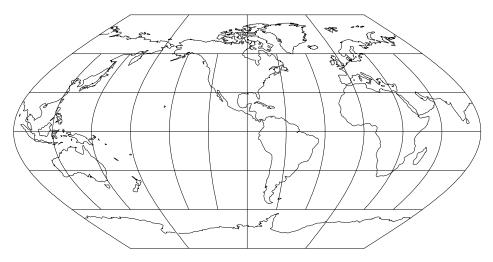
Figure 21: Eckert V projection, with shorelines and 30° graticule. Central Meridian 90° W (+proj=eck5 +lon\_0=90w).
