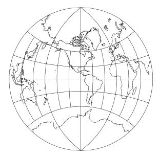
Figure 67: Van der Grinten II projection, with shorelines and 30° graticule. Central Meridian 90° W (+proj=vandg2 +lon\_0=90w).
