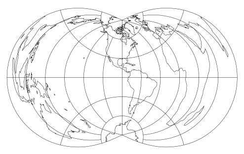
Figure 43: Rectangular Polyconic projection, with shorelines and 30° graticule. Central Meridian 90° W (+proj=rpoly +lon\_0=90w).
