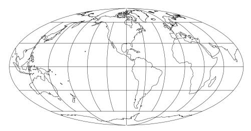
Figure 15: Mollweide projection, with shorelines and 30° graticule. Central Meridian 90° W (+proj=moll +lon\_0=90w).
