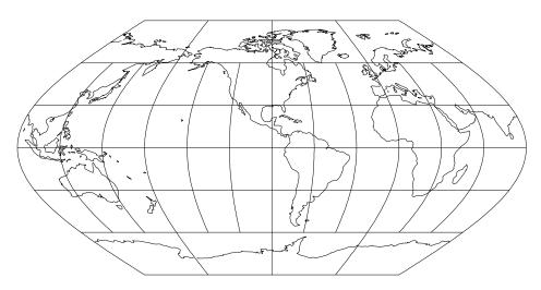
Figure 32: Winkel I projection, with shorelines and  $30^{\circ}$  graticule. Central Meridian  $90^{\circ}$  W (+proj=wink1 +lon\_0=90w).
