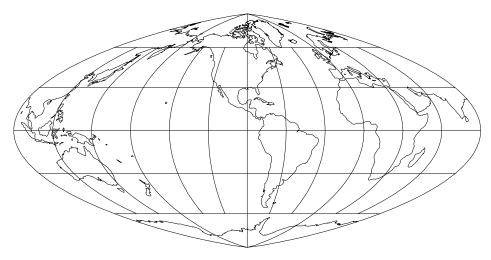
Figure 33: Boggs Eumorphic projection, with shorelines and 30° graticule. Central Meridian 90° W (+proj=boggs +lon\_0=90w).
