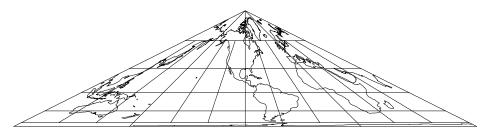
Figure 34: Collignon projection, with shorelines and 30° graticule. Central Meridian 90° W (+proj=collg +lon\_0=90w).
