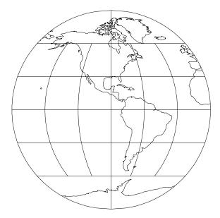
Figure 63: Apian Globular I projection, with shorelines and 30° graticule. Central Meridian 90° W (+proj=apian +lon\_0=90w).
