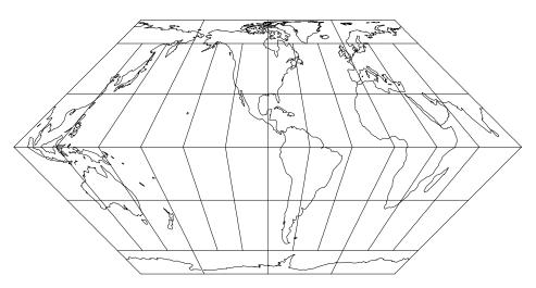
Figure 18: Eckert II projection, with shorelines and 30° graticule. Central Meridian 90° W (+proj=eck2 +lon\_0=90w).
