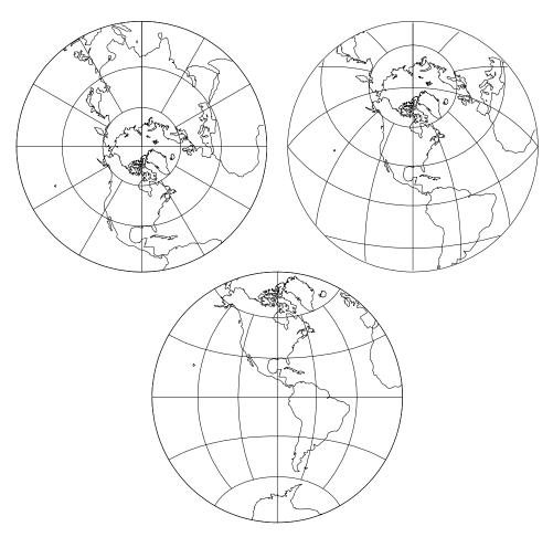
Figure 50: Polar (+lat\_0=90), oblique (+lat\_0=45) and equatorial aspects of the Airy projection, with shorelines and 30° graticule. Central Meridian 90° W and  $\phi_b = 90^\circ$ . (+proj=airy +lon\_0=90w)
