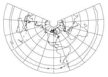
Figure 38: Equidistant Conic projection, with shorelines and  $30^{\circ}$  graticule. Central Meridian  $90^{\circ}$  W. and standard parallels at  $20^{\circ}$  N and  $60^{\circ}$  N (+proj=eqdc +lon\_0=90w +lat\_1=20n +lat\_2=60n).
