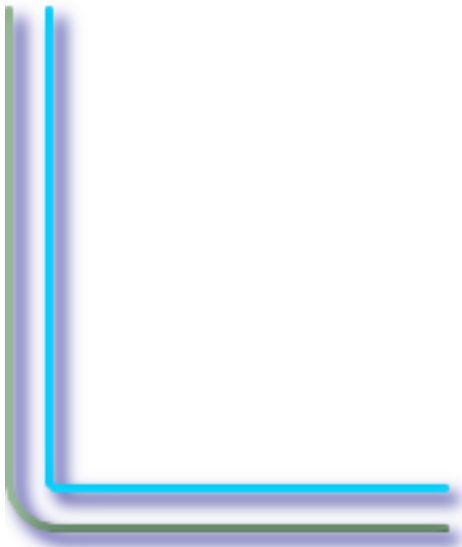
15, 'quad_segs=4 join=round' original line and its offset 15 units.
